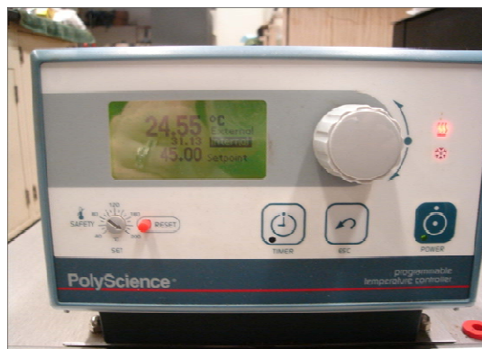
Figure A25 Temperature controller and the power switch of ITS
