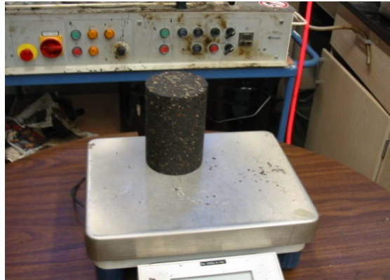
Figure A3 Weight of the sample in dry condition
